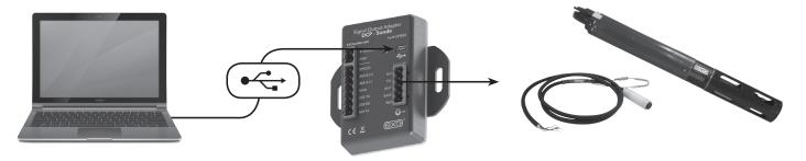
Note: USB utilizes Communication Device Class (CDC) and installs as comport on PC: "YSI SOA/DCP Gen2". The USB connection may also be used to update firmware on the adapter using KOR software.
