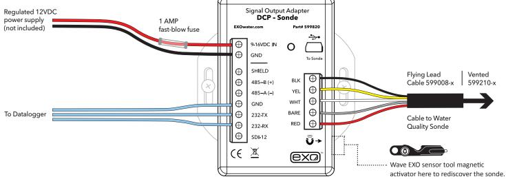
When connecting new sondes to the DCP adapter, it may be necessary to redetect the sonde. This can be done by power cycling the adapter or by using the magnetic read switch at the lower right hand side of the enclosure. Waving the magnet in the EXO sensor tool, over the area referenced by the square above, will force a network redetect where all new sensors and configurations will be discovered.
